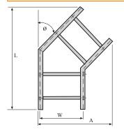
The 60° fitting is fabricated with the horizontal adjustable splice plates.
