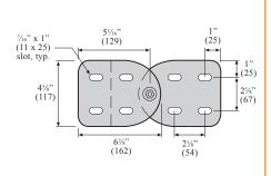
For adjustable vertical plate hardware, use catalog number 505168SS. For travel dimensions, contact us.
